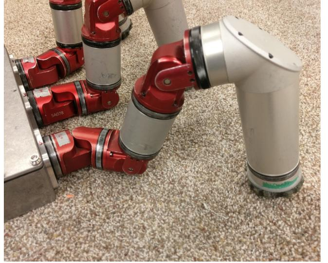
Fig. 3: Hexapod leg joint configuration.
