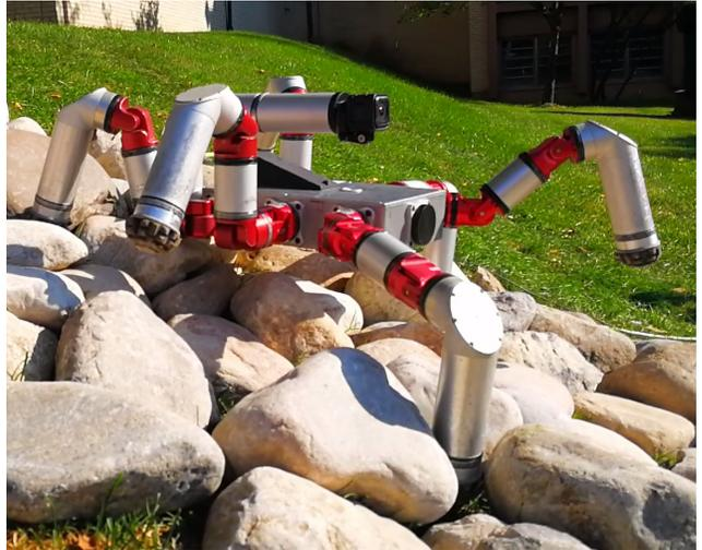
Fig. 1: Hexapod robot climbing down a rocky slope. The mounted camera is only used for point-of-view video recording.
