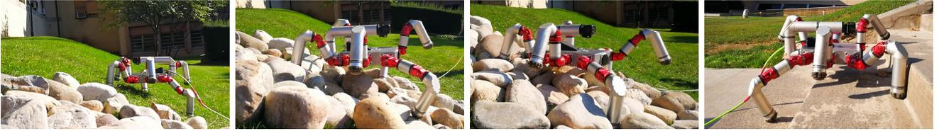
Fig. 7: Sequence of frames of the hexapod robot locomoting through various environments. Using our approach, the robot is able to climb steep grass (around 20 degrees), climb down a similarly-steep rocky slope, and climb up stairs. Full video: <https://goo.gl/awwYfT>
