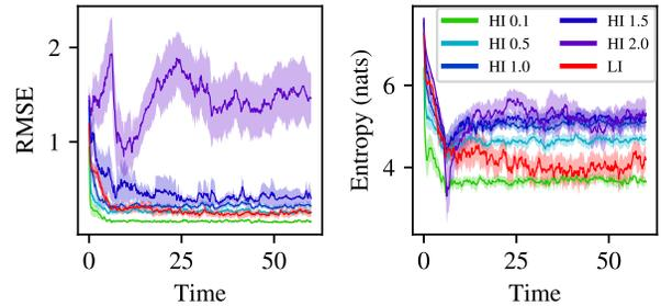
Fig. 5. **Comparison with high information sensors.** (Left) RMSE  $\pm$  2 SE for both higher-information sensors with **B-ETO** (HI) and low-information sensor with **MI-ETO** (LI). The number next to HI is the value of  $\sigma^2$ . (Right) Entropies  $\pm$  2 SE for high and low information sensors. Using **MI-ETO** with a low-information sensors starts to outperform **B-ETO** with the higher-information sensors at around  $\sigma^2 = .5$ .
