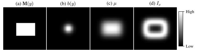
Fig. 2. **Components for calculating the mutual information map.** (a) Sensor footprint mask  $M(y)$  for a rectangular sensor footprint, (b) Current belief about target location  $b(y)$ , (c)  $\mu(x)$  calculated using Equation 16 (shown projected onto  $\mathcal{Y}$ ), (d)  $I_x(y; z)$  calculated using Equation 9 (shown projected onto  $\mathcal{Y}$ )
