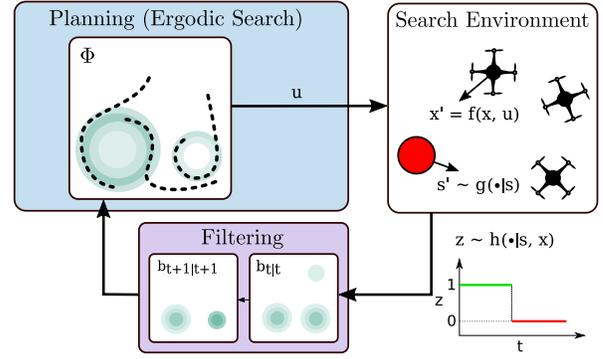
Fig. 3. **ETO pipeline for target search.** The ergodic search algorithm is initialized with a uniform information map  $\Phi$  which is used to provide an initial exploratory control signal to the agents subject to the optimization described in (5). Subsequent binary sensor measurements acquired through exploration are used to filter the belief over the targets which is used to reconstruct  $\Phi$  according to Eq. 9.
