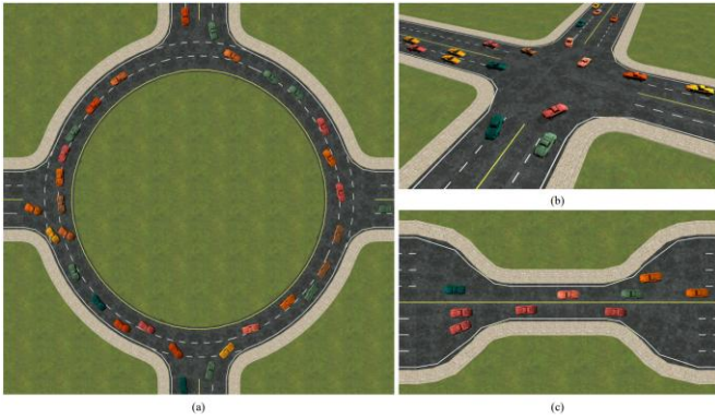
Fig. 3. Illustration of three typical highly interactive and dense traffic scenarios for MASD systems in the MetaDrive simulator: (a) roundabout (left), (b) intersection (up right), and (c) bottleneck (bottom right).
